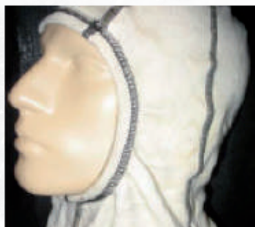
Hood inside out – this side with Nomex® Nano Flex
