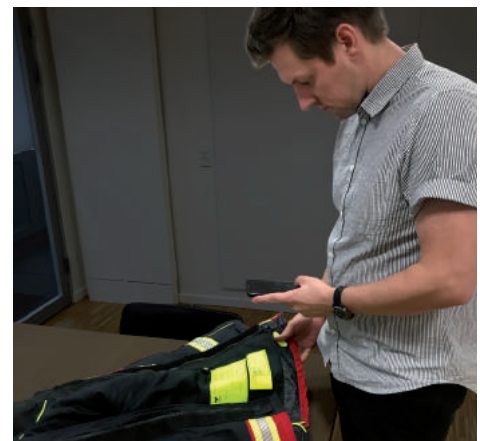
The user scans the bar code or NFC chip and enters the new information about the suit in the app.
