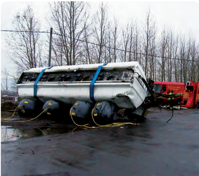
Efficient lifting of overturned vehicles.
